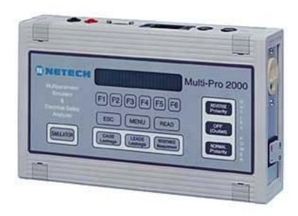
**MULTI-PRO 2000,** Electrical Safety Analyzer is a microprocessor based, full function electrical safety analyzer with a builtin 12 lead ECG Simulator.
