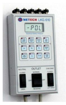
The LKG 610, Electrical Safety analyzer is designed to test any piece of medical equipment. The full featured analyzer is microprocessor controlled and has a full set of ten leads.
